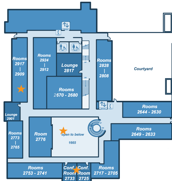
Figure 1: Scanner placement in the building. During the study, BLE scanners were placed in the first floor atrium and in an office and conference room on the second floor.
